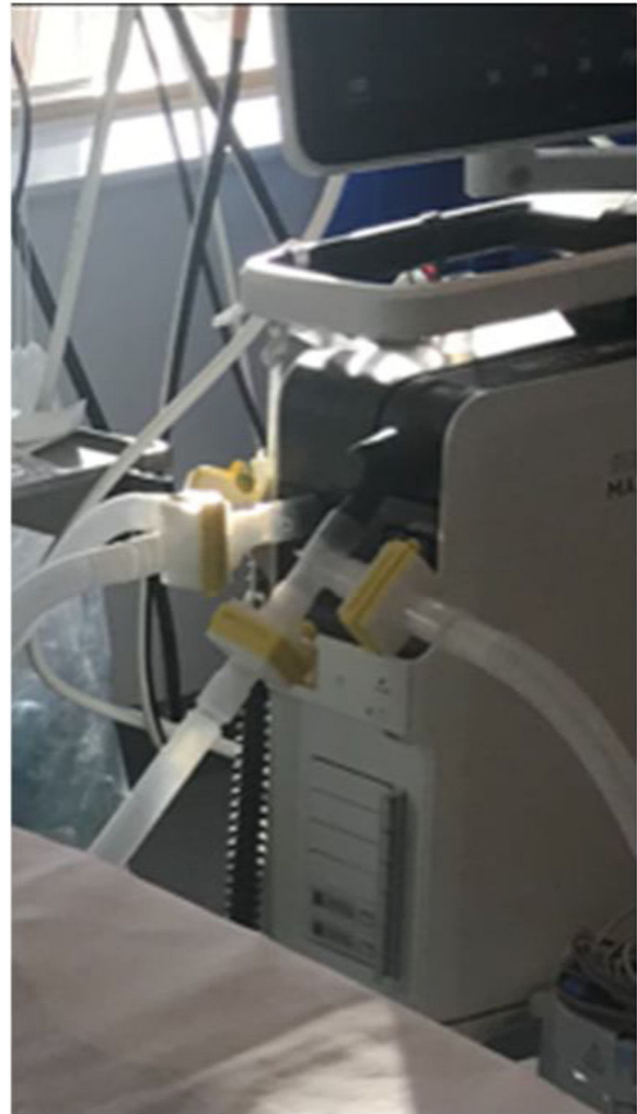
Figure 1 Two sets of standard ventilator tubing (Hudson) were connected to a single ventilator (tested in each model of ventilator, Puritan-Bennett, 840 series and a Servo I Maquet) via two T-tubes (one on the patient inflow limb of the circuit, and one on the patient exhaust limb). Each T-tube was attached to a microfilter (total of four) to isolate both patients and the ventilator. Especially if the circuit do not have in place non-return valves.
